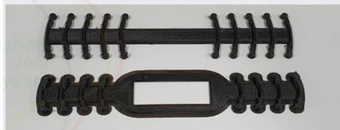
A 3D Printed Ear Guard for Comfortable Use of Face Masks by Healthcare Workers
